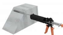
Feed the hole from the end to the external surface by going back from 1 mixer graduation between each pump.
