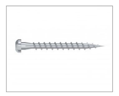
CSA connector screw is developed for installing Simpson Strong-Tie connectors to timber, in order to obtain the published load bearing capacities. The conical shape under the head ensures a full contact with the connector which increases the transfer of force. A fixed connection with larger cross-bearing capacity than for standard screws is obtained. The 6 lobe recess helps to fix the screw during insertion.
