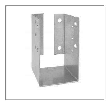
Joist Hangers especially developped for glulam application. It can be installed on timber or concrete support with bolts only and can be manufactured for large dimension of timber joist.
