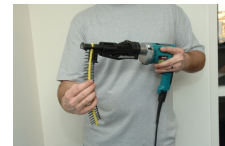
Insert the tape screw tip pointed up: your screwdriver is ready!
