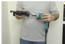
Engage the gun with the mandrel and snap it onto the adapter.
