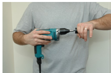
Remove screw driver sleeve.
