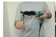
Insert the tape screw tip pointed up: your screwdriver is ready!
