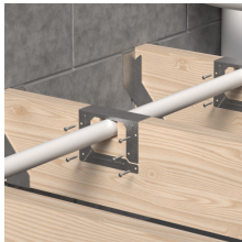
Step 4: Bend the relief tab inwards against the joist and fasten the bracket using 5 screws (included with the kit) into the face of the joist.
