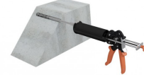
Fill the hole to half or two thirds. Withdrawing the nozzles with each pump.
