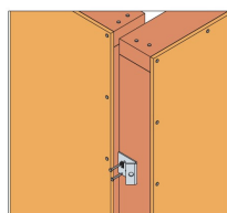
Corner Panel Installation: Install the Square Twist Nails
