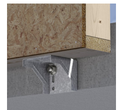
Bracket below, in the middle of concrete
