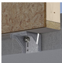
Bracket below, in the middle of concrete
