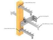
*Fix the insulation by mounting ABMI claws on ABC brackets*
